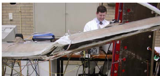
Figure 1: The view of the Trailing Edge of Blade 9 and the principal author immediately after blade failure
