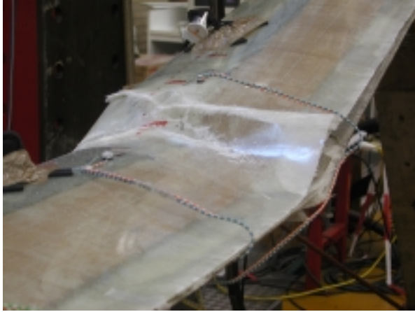
figure 12: Blade fractured in static loading at the defect zone
