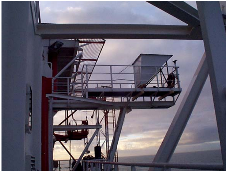
Figure 6-2: SODAR located at MPN as seen from below (without cuffs).
