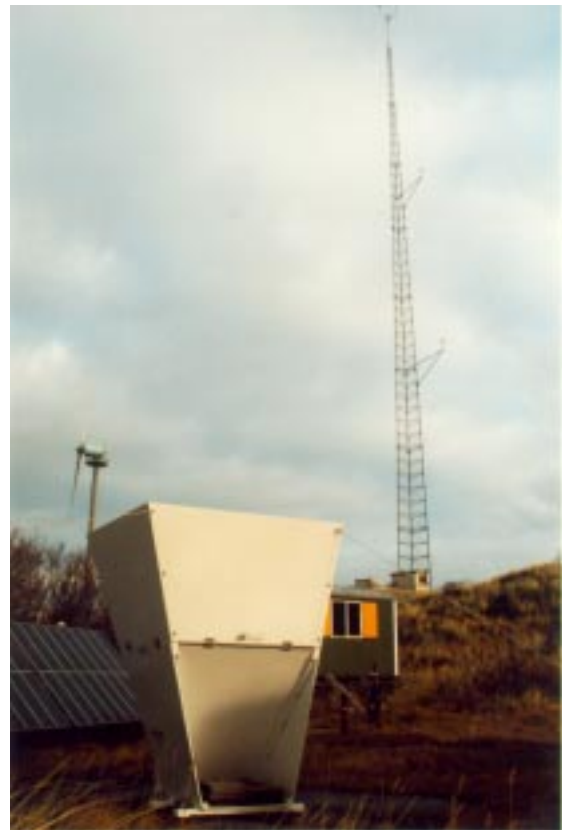
Figure 2: SODAR at the ECN wind turbine test site
