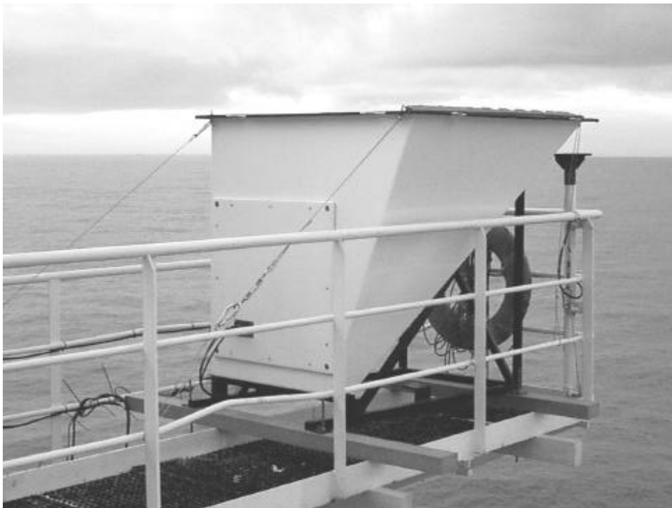
Figure 5 View of the mini-SODAR equipment installed at Measuring Post Noordwijk offshore research platform
